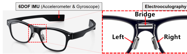
Figure 2: The Jins Meme smartglasses and its EOG sensor placement. The IMU is at the end of the right leg.
