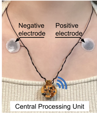
Figure 8: Demonstration of wearing the ECG Necklace (without any fashion decorations).
