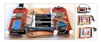
Figure 3: Left: The AdHocProx prototype hardware consists of two ESP32 microcontrollers, two DW3000 UWB radios, and four capacitive touch sensing electrodes. Right: The AdHocProx attachment on three devices with different form factors: Microsoft Surface Duo dual 5.6" screen smartphone, 10" Microsoft Surface Go and 12" Microsoft Surface Pro 7.
