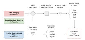
Figure 6: Sensor processing block diagram.
