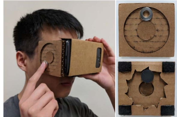
Figure 1: ScratchVR is a low-cost technique for mobile VR headsets, such as Google Cardboard, to expand the interaction space by introducing bidirectional scrolling using a click wheel design. (a) User interacting with ScratchVR; (b) Spinning washer is used as the human interface; (c) Magnet in the inner cardboard layer slots into place for more reliable recognition and haptic feedback.
