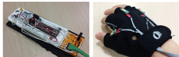
Figure 1. Tactile Teacher Prototype with a microcontroller (left) directly connected to an instrumented glove (right)
